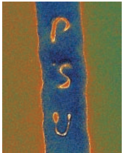
A silicon nanowire, 40nm in diameter, etched by a beam of finely focused high intensity electrons. This work was performed by Drs. Moses Chan, Shenyong Xu and Joan Redwing at Penn State University.
